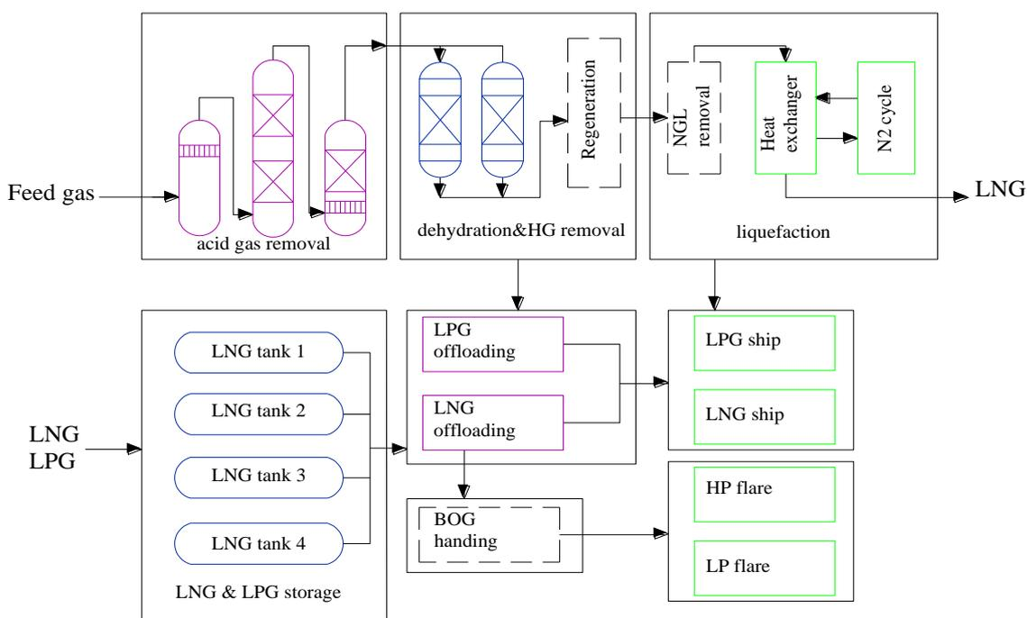
FIGURE 1 Flow diagram of production, storage and unloading device of FLNG unit
